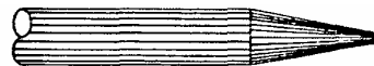
RIGHT: lengthwise grind marks don't restrict Current. Mirror finish is even better.
