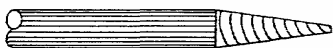
WRONG: crosswise grind marks restrict welding Current, cause arc wander, risk inclusions.
